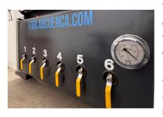
The CNC router we worked with has a vacuum table divided into six independent sections, controlled by valves. Each section can be activated or deactivated depending on the size and position of the material being cut. By closing certain valves and keeping only the necessary sections open, we could optimize the suction force applied to the board, making sure it stayed completely flat against the sacrificial board.
